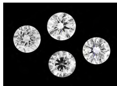
Figure 14. These four near-colorless round brilliant melee were identified as HPHT synthetic diamonds lacking the typical Si- and Ni-related defects.
