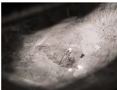
Figure 11. Under reflected illumination, the pink sapphire's large cavity filling was readily visible with the unaided eye. Field of view 2.70 mm.
