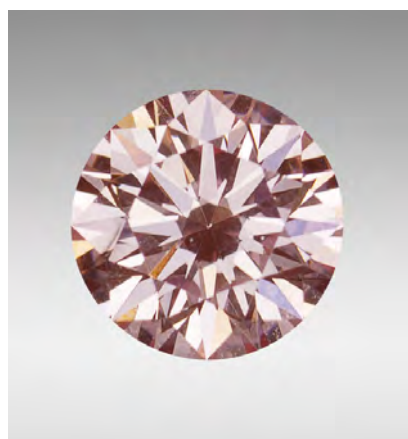
Figure 12. This 0.26 ct pink synthetic diamond contains the first H4 defect GIA has observed in a CVD synthetic diamond.
