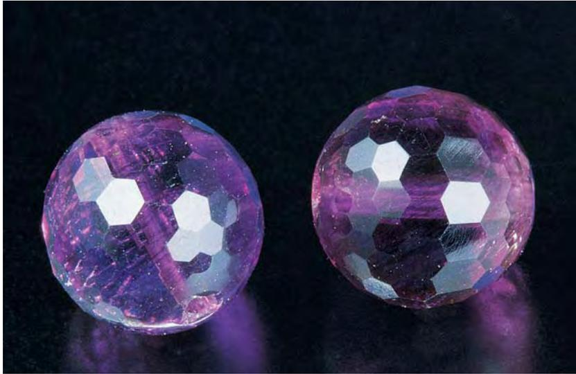
Figure 11. These purple beads, each about 10 mm in diameter, were offered as amethyst. They are actually colorless quartz that has been quench-crackled and dyed purple.
