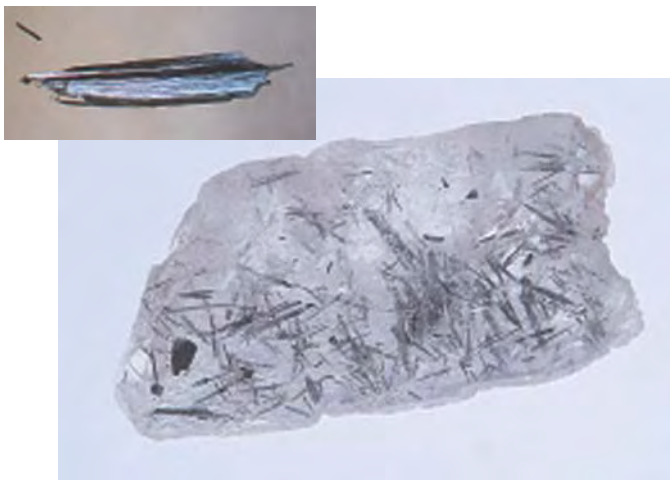
Figure 11. Metallic gray inclusions of pääkkönenite in quartz have been recovered from the Cryo-Genie mine, as shown by this sample (1.8 cm long; GIA Collection no. 30485) donated by Gochenour's Minerals; photo by Maha Tannous. The inset shows one of the inclusions in more detail; photomicrograph by John I. Koivula, magnified 10×.
