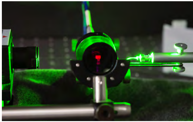
Figure 2. With a green laser beam illuminating it from the left, and a color filter positioned in front to remove green light, an emerald crystal (center) is seen to emit red photoluminescence. Photo by D.B. Thompson.
