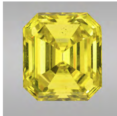
Figure 7. This 59.88 ct Fancy Vivid yellow diamond was treated through artificial irradiation and annealing.
