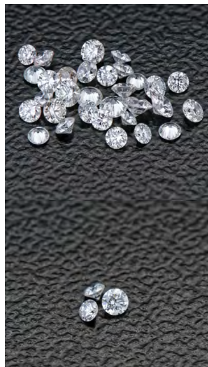
Figure 23. From an initial screening of 3,005 melee diamonds, 24 specimens were referred for further testing. Of these, three were HPHT-grown synthetic diamonds.
