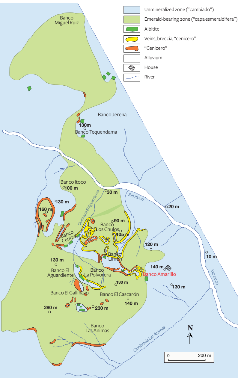
Figure 5. Geological map of the Muzo mines, with the height of each mining site reported in bold. Modified from Barriga Villalba (1948).
