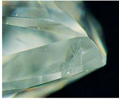
Figure 2. Before processing (left), this fracture in the 0.61 ct GGL sample was bright and reflective. After HPHT processing (right), the area of the original fracture had acquired a coarse (frosted) texture and we noticed the addition of a bright transparent extension, or “fringe.” No graphitization was observed. Photomicrographs by Christopher P. Smith; magnified 55 \times .
