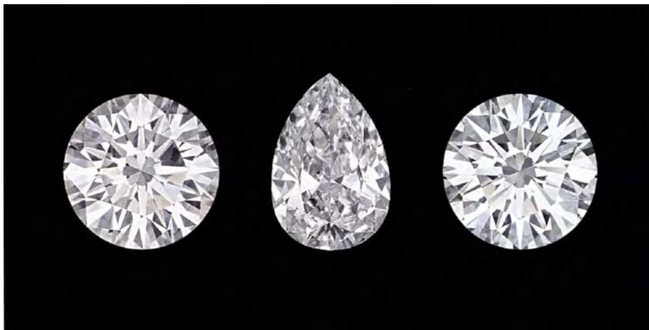
Figure 1. These three diamonds, all from the same manufacturer, were studied to determine which two, if any, were cut from the same piece of rough. All of the diamonds were graded as E color and VS 1 clarity. Sample A (left) weighs 1.08 ct, sample B (center) is 0.81 ct, and sample C (right) weighs 1.05 ct. Samples B and C were proved to originate from the same rough diamond.
