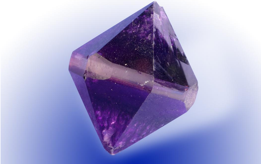
Figure DD-1. This \text{NH}_4\text{F} -grown synthetic amethyst crystal weighs more than 600 g. These crystals are grown using basal seed plates, and show excellent coloration. Such \text{NH}_4\text{F} -grown synthetic amethysts are rare. Photo by Alain Cossard.
