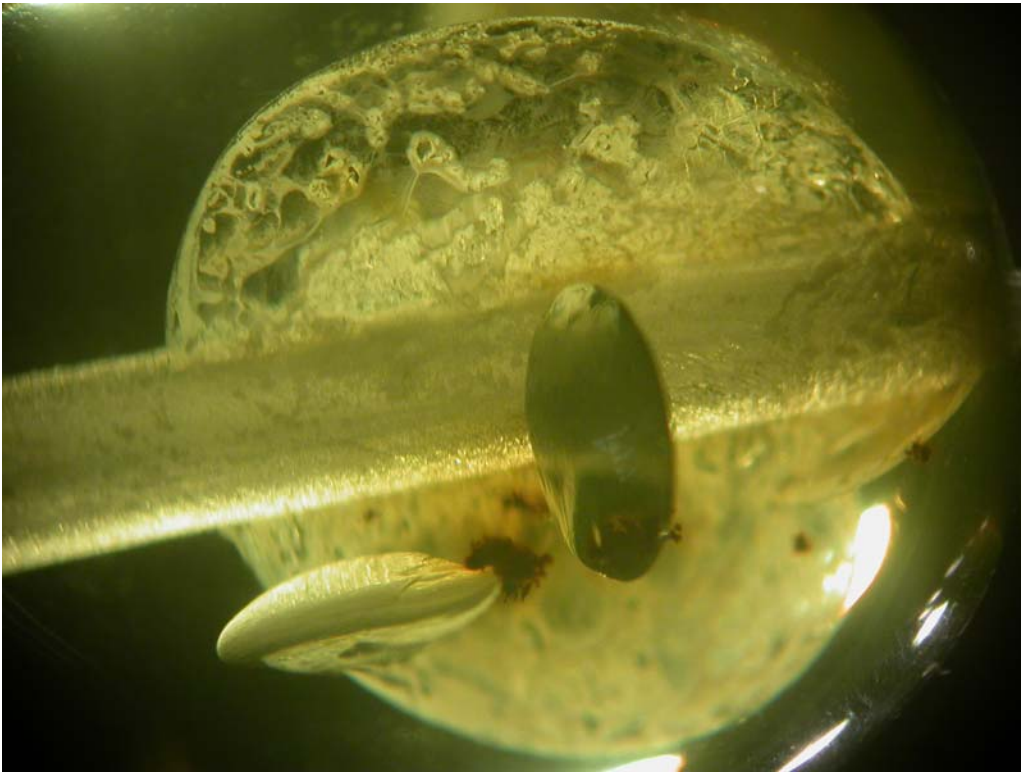
Figure DD-2. “Sun spangles” were created through the one- and two-stage heating processes of copal and amber. These features are formed by cracks surrounding small air bubbles or other contamination.. Photomicrograph by A. Abduriyim; magnified 20x (sample TR-001).
