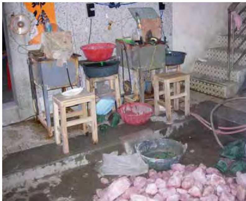
Rose quartz and jade are processed in this workshop in Hai Feng County, Guangdong Province, China. Ventilation is limited to the small wall-mounted fan on the left. Note also the exposed belts and pulleys on the drive motors, and the loose electrical cables sharing space with water hoses. Photo courtesy China Labor Bulletin.
