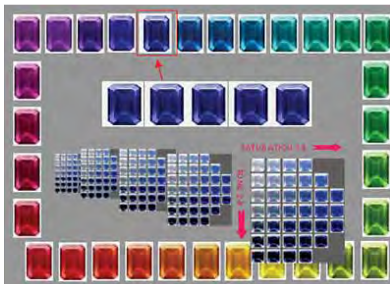
The main screen of this computerized system designed for color communication (Gemewizard software) displays 31 master hues. Tonesaturation grids were developed for each hue, as shown here for blue.
