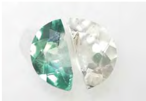
This 5.57 ct “diffused” (coated) topaz is shown before (left) and after (right) immersion in hydrofluoric acid. Photo by Min Htut.
