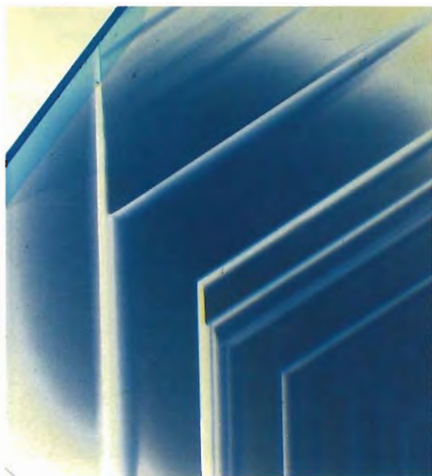
Figure 7. One of the most obvious ways to identify sharpened growth structures is through color zones, or bands, the thickness of which may fluctuate between consecutive periods of crystal growth. Shown here are broad blue color bands alternating with narrow colorless bands, parallel to dipyrnidal v ( 44\bar{8}3 ) planes, in a sapphire from Kashmir. The vertical growth planes are at 15.4^\circ from the optic axis direction, and the angle created at the junction of the v - v planes is 123^\circ . Immersion, magnified 15\times .
