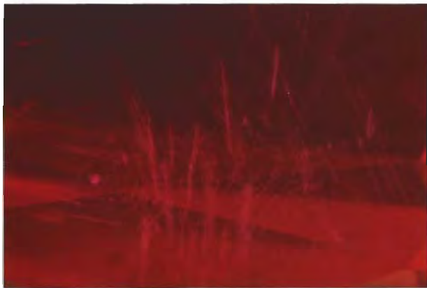
Figure 12. "Antennae-like" stringer formations, a typical feature of Vietnamese rubies, helped confirm that the 4.51 ct stone was natural. Oblique fiber-optic illumination, magnified 22 \times .
