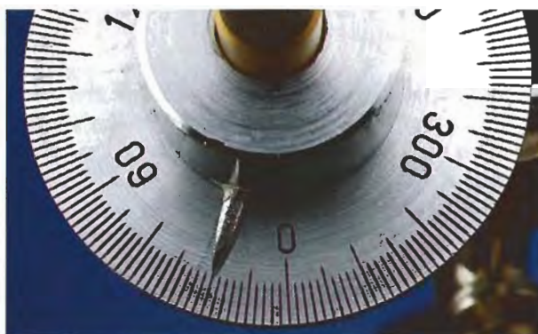
Figure 8. By rotating the stone holder until the growth features are sharply defined, the pointer will show the number of degrees, on the indicator dial, that the growth features are located from the optic-axis direction. The measurement of 20 shown here identifies a series of dipyrnidal w ( 11\bar{2}1 ) planes, which are located characteristically at 20.1^\circ from the optic-axis direction. Photo by Shane F. McClure.
