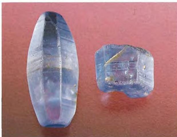
Figure 2. The external form, or habit, of a crystal is made up of a collection of various crystal faces. The number and relative prominence of these crystal faces can have a significant influence on the overall shape of the crystal. Shown here are bipyramidal (left) and tabular (right) blue sapphire crystals from Sri Lanka. The line diagrams illustrate which crystal faces comprise the habits of these two crystals: the basal pinacoid c (0001), the positive rhombohedron r ( 10\bar{1}1 ), the hexagonal dipyramid w ( 11\bar{2}1 ), and the second-order prism a ( 11\bar{2}0 ). Photo by Shane F. McClure.
