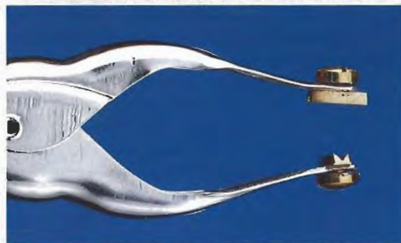
Figure A-2. The author's modification to the basic stone holder consists of two independently rotating grooved channels, which allow for an additional rotation capability so that the c-axis remains in a vertical position. Photo by Shane F. McClure.
