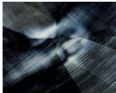
Figure 17. When viewed with cross-polarized light, most of the GE POL diamonds exhibited banded (left) or crosshatched (center and right) strain patterns. Although some stones did reveal low-intensity interference colors (right), for the most part these diamonds showed moderate- to high-intensity interference colors (center and left), notably stronger than what is normally seen in untreated diamonds of similar color. Left and center photomicrographs by Shane F. McClure, magnified 20×; right photomicrograph by John I. Koivula; magnified 20×.
