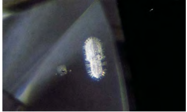
Figure 13. This small solid inclusion surrounded by a stress crack is an example of a feature seen in 103 of the GE POL diamonds. Photomicrograph by Vincent Cracco; magnified 63 \times .
