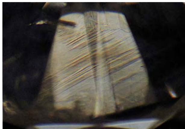
Figure 9. Also observed was brown graining, often in a parallel banded pattern. Photomicrograph by Shane F. McClure; magnified 40 \times .
