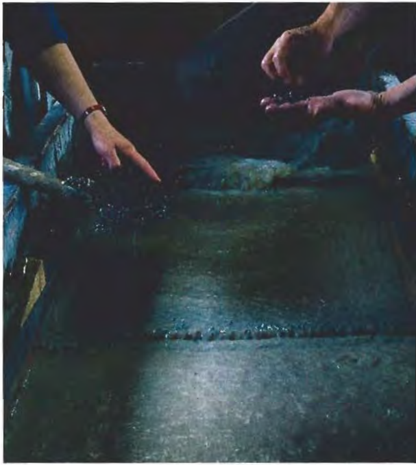
Figure 5. Density separation is used to concentrate the pyropes in this jig at Podsedice. Photo by J. Schlüter.
