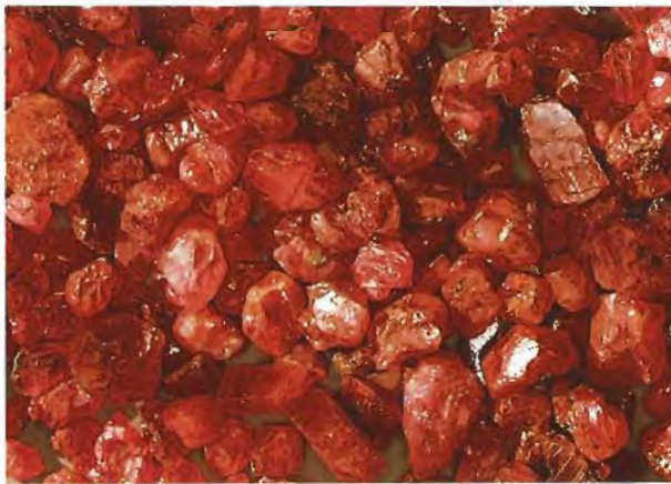
Figure 3. These ruby crystals were sorted from parcels of rough spinels that were reportedly from the relatively new find at Morogoro. The largest pieces are approximately 20 ct. Photo by H. Hänni.
