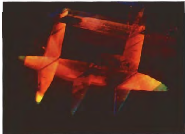
Figure 8. The Morogoro rubies frequently exhibited narrow twin lamellae oriented parallel to one or more rhombohedral faces. Here, two systems of lamellae intersect. Immersion, crossed polarizers, magnified 25 \times ; photomicrograph by K. Schmetzer.
