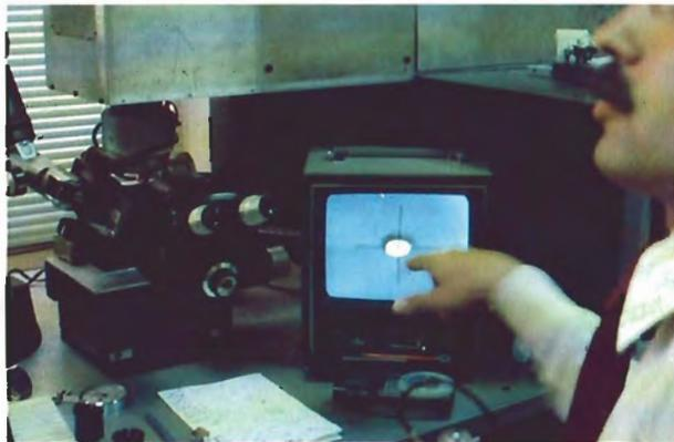
Figure 2. To complete the laser saw unit, this figure shows the x-y platform, the focusing lens, and the microscope and television monitor used to observe the progress of the laser through the stone.
