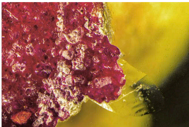
Figure 5. Tool marks from a rotary abrasive burr are clearly visible in this manufactured floral-shaped inclusion (left; field of view 9.72 mm). The cavity was subsequently filled with a yellow and red composite material consisting of sand grains and a colored binder or resin material (right; field of view 4.26 mm). Photomicrographs by Nathan Renfro; courtesy of Mike Bowers.
