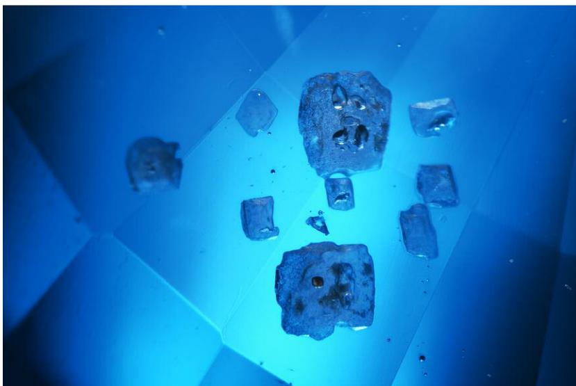
the refractive index liquid, the stone's specific gravity and doubly refractive nature point to sapphire. Advanced testing was useful in confirming the true identity of the stone and the coating.
