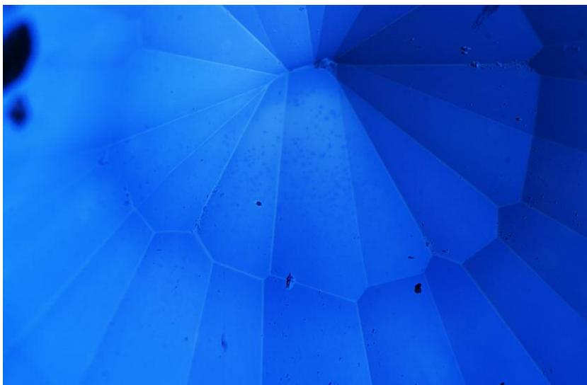
*Figure 12. Lighter facet junctions and a speckled surface are evidence of coating. Field of view 4.79 mm.*
