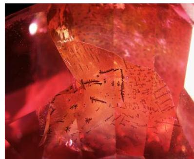
Figure 21. The foreign material partially crystallized in a dendritic pattern in the fractures, reminiscent of diaspore. Field of view 7.64 mm.
