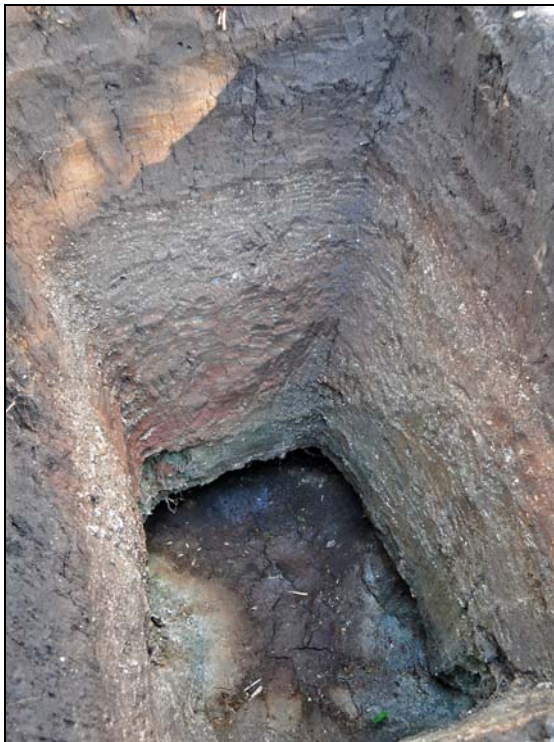
Figure 37: Details of typical mining pits (about 4 to 8 meters deep) near Namahumbire, the numerous pits have already been damaged by the arrival of the rainy season at the end of November and will soon be flooded. Photo V. Pardieu / GIA Laboratory Bangkok, December 2009.
