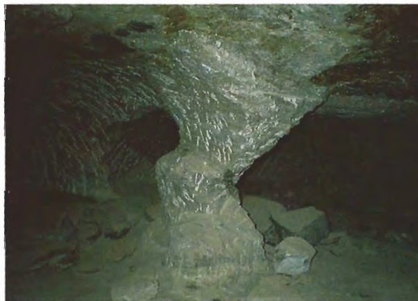
Figure 8. This view is inside one of the mines on the north wall of Wadi Zabara, entered through a near-vertical shaft excavated along the schist-gneissic granite contact. Note the chisel marks and the pillar, approximately 1 m in diameter, left as support. Photo by Robert C. Kammerling.
