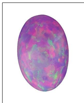
Figure 1. This 5.90 ct hydrophane-type opal showed gemological features consistent with material from Wollo Province, Ethiopia. The purple color proved to be caused by dye. Photo by Robison McMurtry.
