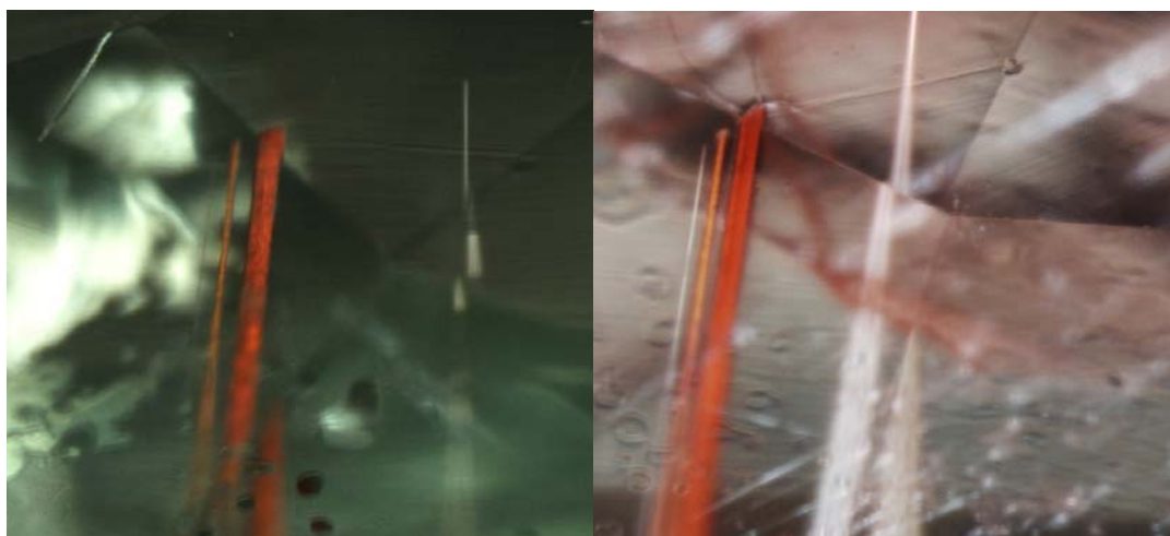
Figure 15: Sample 0668227002 comparable areas before (left) after heating at 700°C in air for 10 hours (right); no foreign elements were added before or during the heating process. In the right-hand image it can be seen that the color within the channel is more even and is slightly more towards orange; also a purplish-pink color has appeared within a fracture to the right of the channel.
