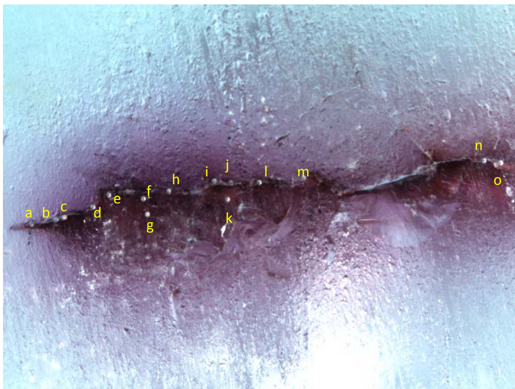
Figure 83: Photomicrograph of the spots analyzed by using LA-ICP-MS after the stone had been ground down 0.5 cm. Each spot was analyzed at the ground down surface (first number in the following pairs for each spot) and 2 \mu m below the surface (second number in the following pairs for each spot).
