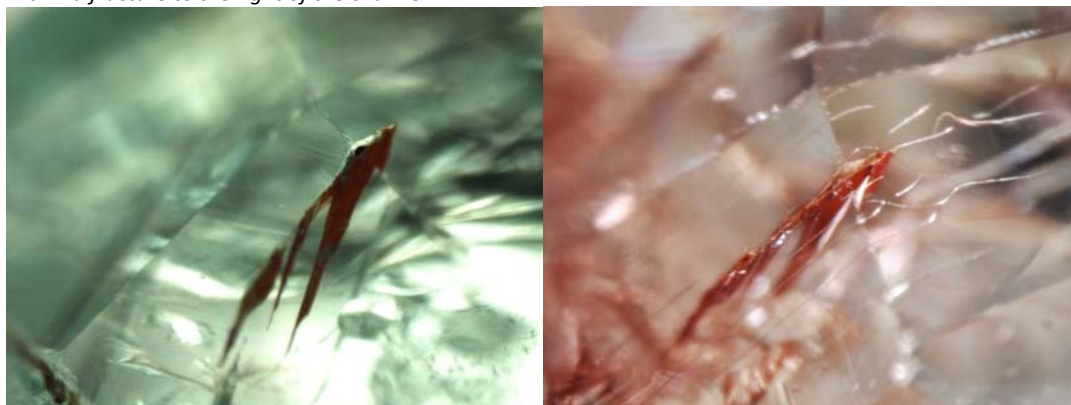
Figure 16: Sample 0668227002 comparable areas before (left) after heating at 700°C in air for 10 hours (right); no foreign elements were added before or during the heating process. (see Figure 17 for a closer study).
