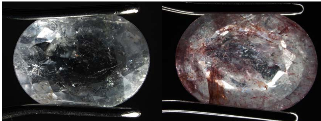
Figure 21: Sample 0668227202 before (left) and after heating at 700°C in air for 10 hours (right); no foreign elements were added before or during the heating process. The overall color impression has changed following heating from bluish (left) to purplish (right)
