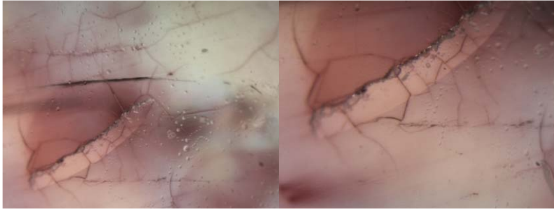
Figure 43: Fine fractures in sample 0668228402 after heating at 700°C in air for 10 hours (left) and at higher magnification (right). See also Figure 42.
