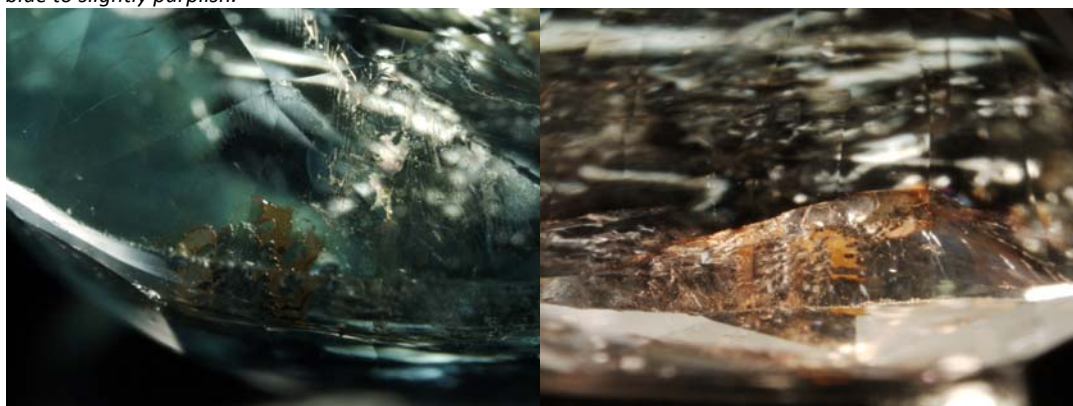
Figure 11: Sample 0668225902 comparable areas before (left) after heating at 700°C in air for 10 hours (right); no foreign elements were added before or during the heating process.
