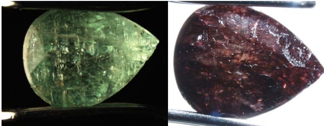
Figure 64: 0668228002 before heating (left) and after heating at 700°C in air for 100 hours ; no foreign elements were added before or during the heating process. The color appearance changed from green before treatment to an intense purplish red after treatment.
