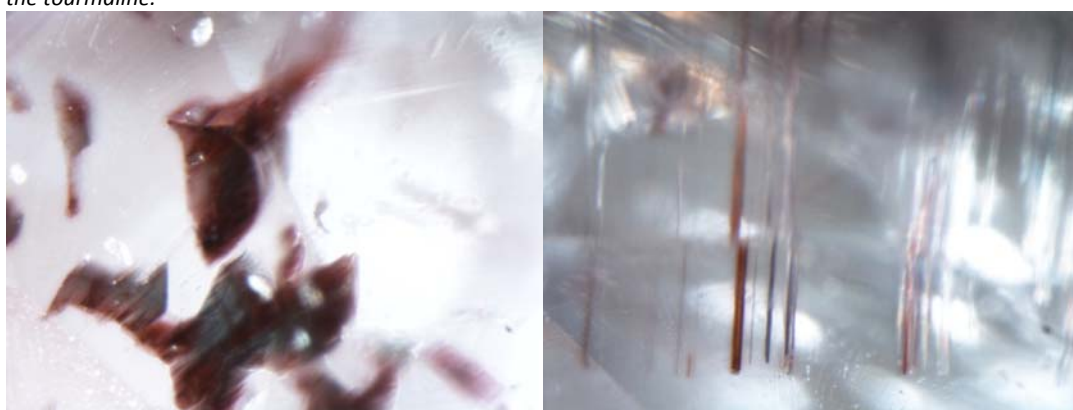
Figure 39: Channels in sample 0668227202 after heating at 700°C in air for 10 hours . In these images, similarly to that seen in Figure 37 and Figure 38, there is a distinct impression that the color in these channels is bleeding into the body of the tourmaline.
