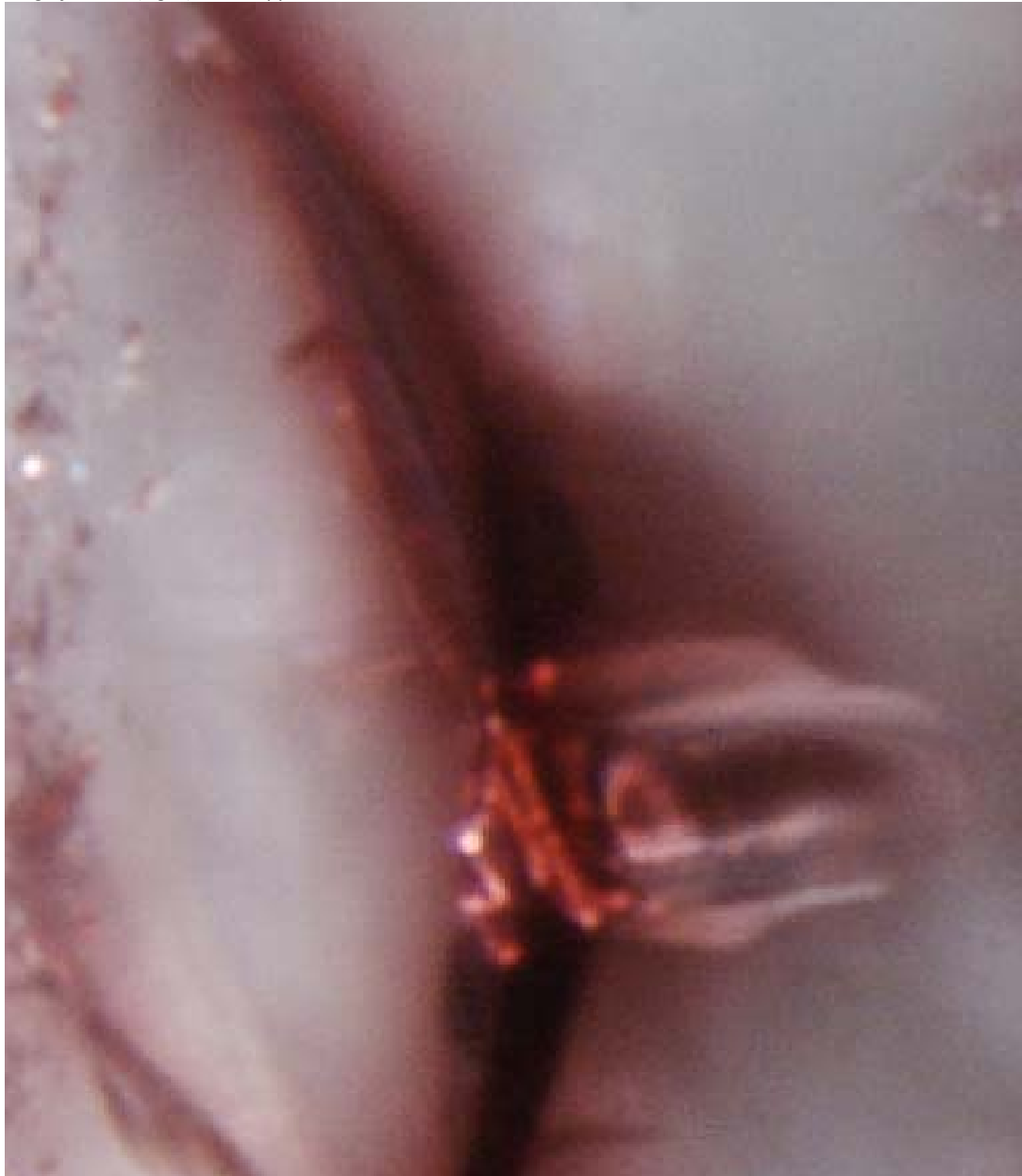
Figure 62: 0668227702 after heating at 700°C in air for 100 hours; no foreign elements were added before or during the heating process. A higher magnification of the fracture seen in Figure 61 (right). The deep reddish brown coloration appears to bleed into the tourmaline host.
