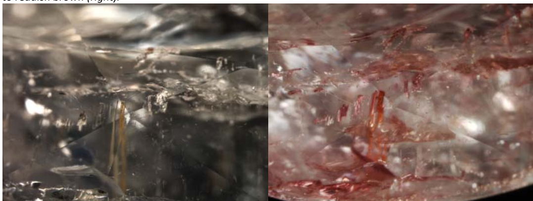
Figure 26: Sample 0668227202 comparable areas before (left) and after heating at 700°C in air for 10 hours (right) no foreign elements were added before or during the heating process (see Figure 27 for a closer study).
