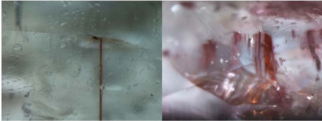
Figure 40: Channels in samples 0668228402 (left) 0668227202 (right) after heating at 700°C in air for 10 hours . In these images, similarly to that seen in Figure 37, Figure 38 and Figure 39, there is a distinct impression that the color in these channels is bleeding into the body of the tourmaline.
