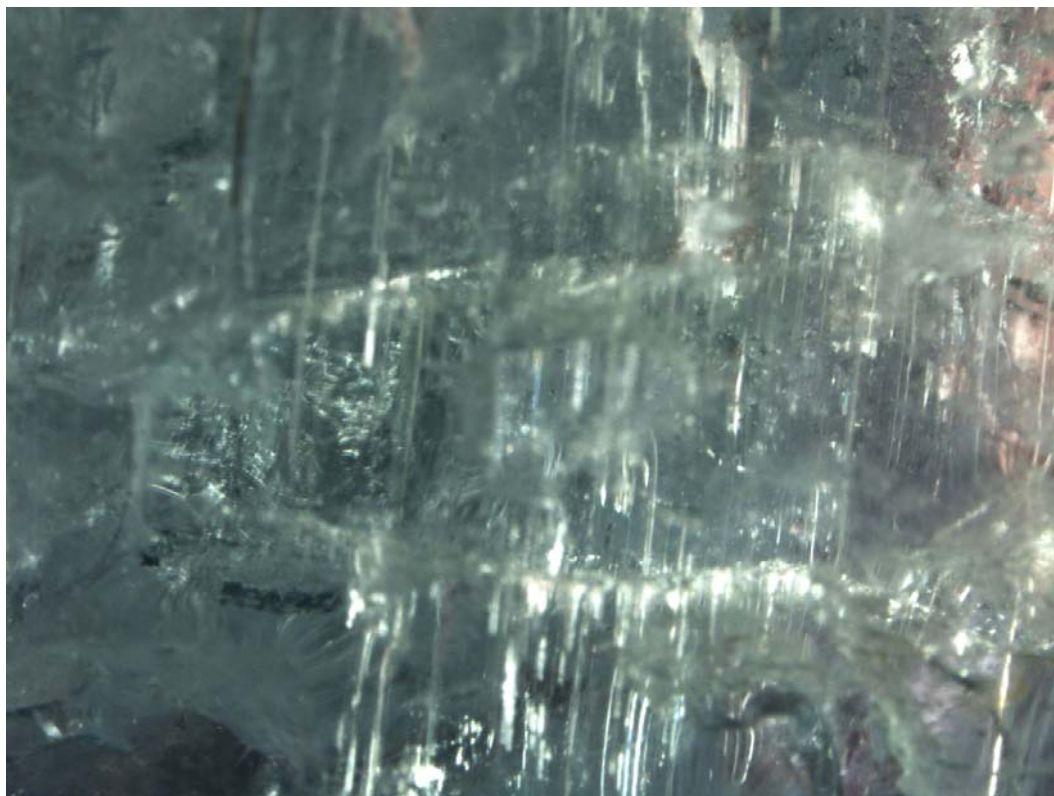
Figure 76: Partially healed fissures and growth tubes in the tourmaline examined for this study
