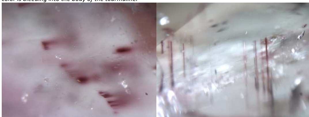
Figure 38: Channels in sample 0668227202 after heating at 700°C in air for 10 hours . In these images, similarly to that seen in Figure 37, there is a distinct impression that the color in these channels is bleeding into the body of the tourmaline.
