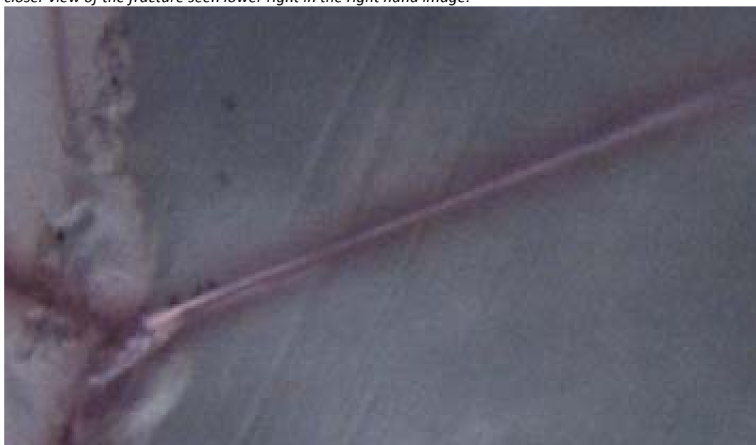
Figure 74: 0668226602 a closer view of the fracture seen lower right in the right-hand image in Figure 73. The purple color is appears to be strongest on the walls of the fracture and then fades into the tourmaline host.
