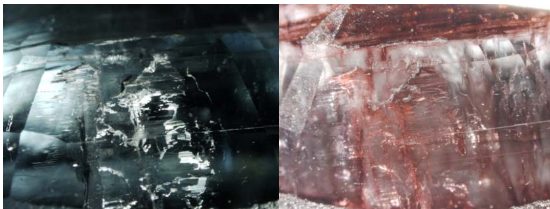
Figure 58: 0668227702 comparable areas before heating (left) and after heating at 700°C in air for 100 hours ; no foreign elements were added before or during the heating process. The partially visible fracture in the center of the image on the left appears reddish brown in the image on the right.
