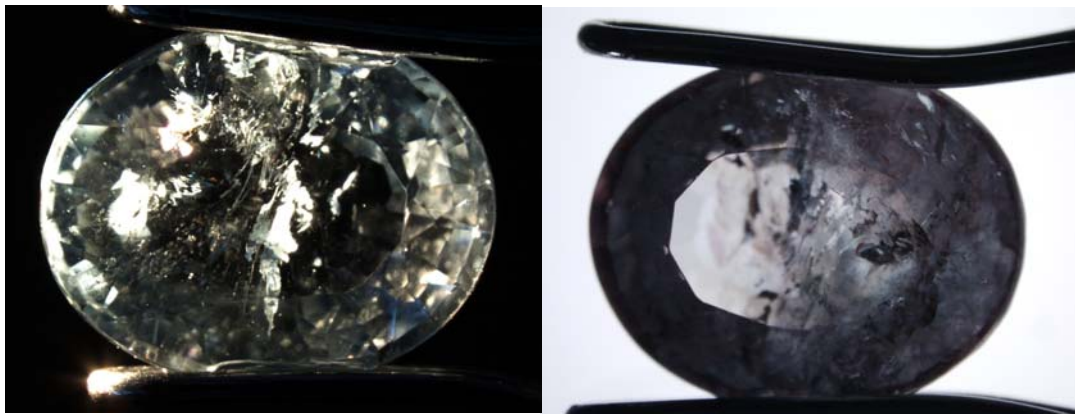
Figure 70: 0668226602 before heating (left) and after heating at 700°C in air for 100 hours ; no foreign elements were added before or during the heating process. Greenish blue before treatment, this stone now has a slight purplish appearance - not as striking a change as previous stones in the group.
