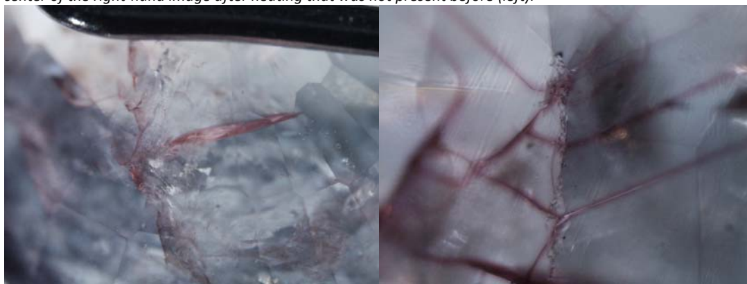
Figure 73: 0668226602 after heating at 700°C in air for 100 hours ; no foreign elements were added before or during the heating process. A purple color is seen to have appeared within several fractures. See Figure 74 for a closer view of the fracture seen lower right in the right hand image.
