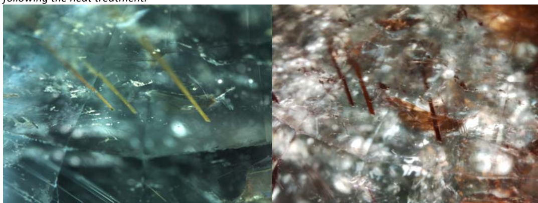
Figure 35: Sample 0668228402 comparable areas before (left) and after heating at 700°C in air for 10 hours (right); no foreign elements were added before or during the heating process. The color of these channels running top left to bottom right has changed from yellowish before heat treatment (left) to a deep reddish brown after (right). A fracture associated with the channel on the right also became reddish brown after heating.
