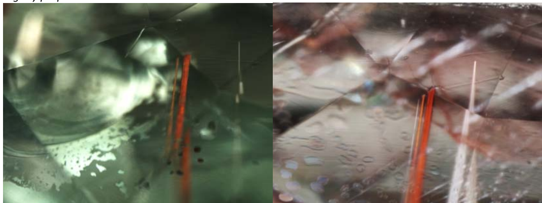
Figure 14: Sample 0668227002 comparable areas before (left) after heating at 700°C in air for 10 hours (right); no foreign elements were added before or during the heating process (see Figure 15 for a closer study).
