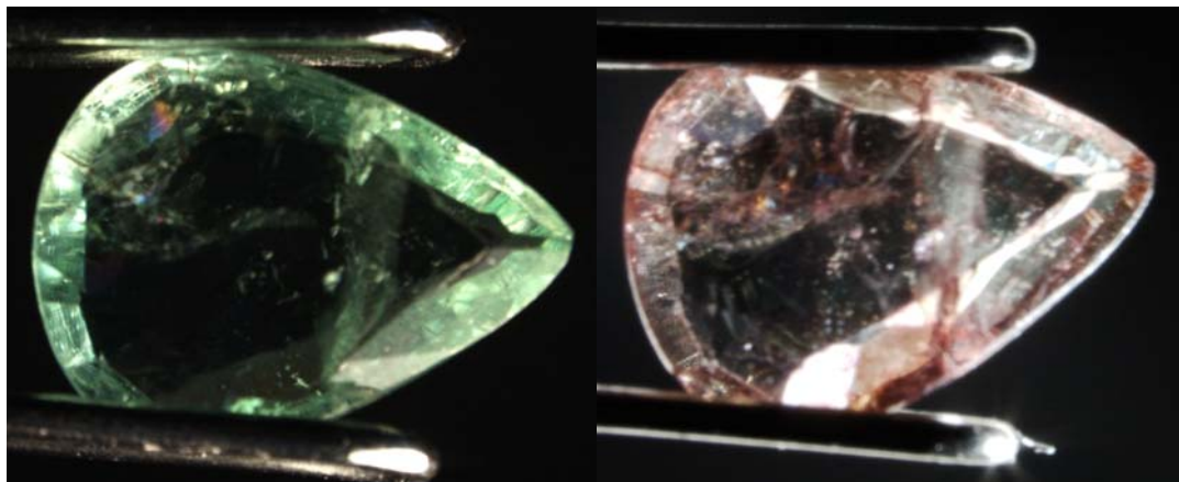
Figure 13: Sample 0668227002 before (left) after heating at 700°C in air for 10 hours (right); no foreign elements were added before or during the heating process. The overall face-up color impression changes from green to slightly purplish.
