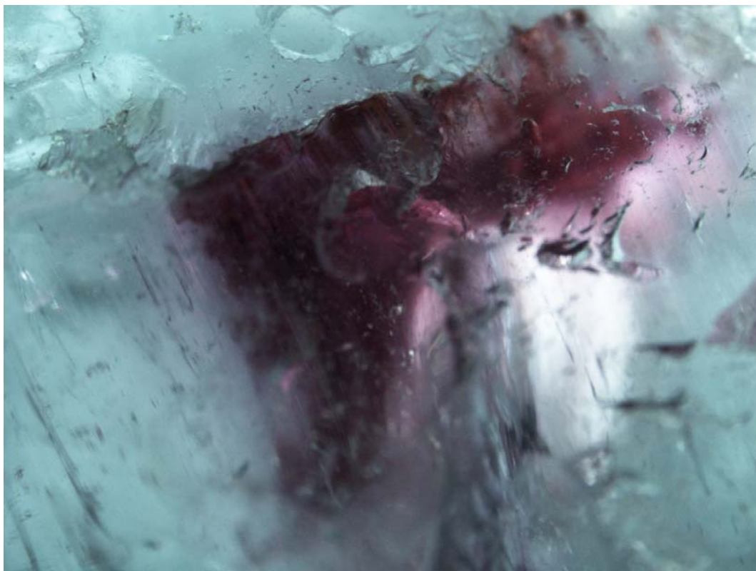
Figure 78: Unusual pinkish purple coloration in growth tubes and cracks in the sample stone.
