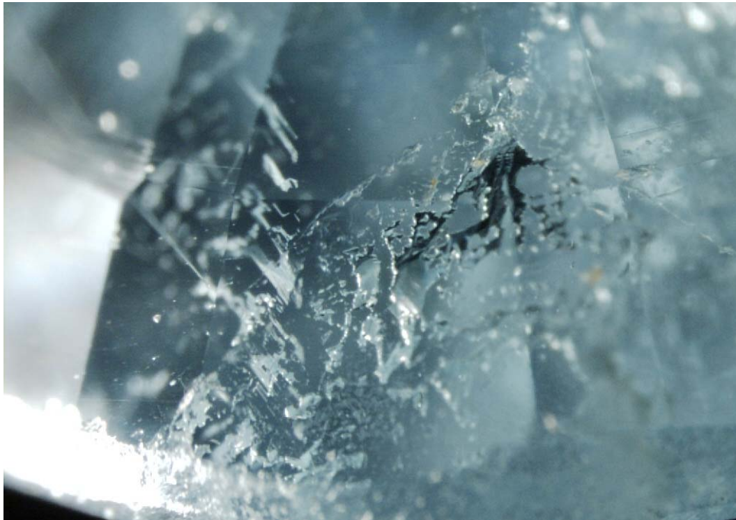
Figure 2: Partially healed fissures in one of the tourmaline selected for diffusion experiments.
