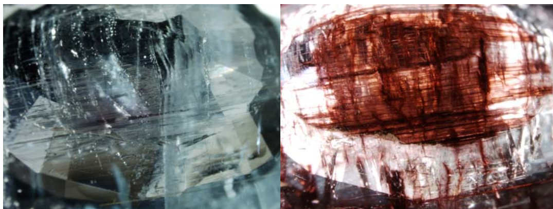
Figure 55: 0668227702 comparable areas before heating (left) and after heating at 700°C in air for 100 hours ; no foreign elements were added before or during the heating process. A large plus numerous smaller fractures appear reddish brown following the heat treatment process, see also Figure 56.
