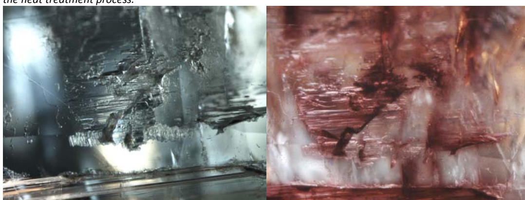
Figure 60: 0668227702 comparable areas before heating (left) and after heating at 700°C in air for 100 hours ; no foreign elements were added before or during the heating process. The partially visible fracture in the center of the image on the left and the fracture running west-east at the bottom of the image appear reddish brown in the image on the right as do several other fractures following the heat treatment process.
