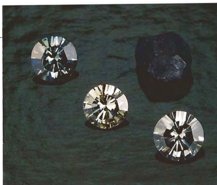
Figure 1. The three small boron-doped faceted synthetic diamonds examined for this study—from left to right, 0.063 ct (sample 2), 0.049 ct (sample 3), and 0.075 ct (sample 1)—and the 0.197-ct crystal were grown at the De Beers Diamond Research Laboratory. Photo by Robert Weldon.
