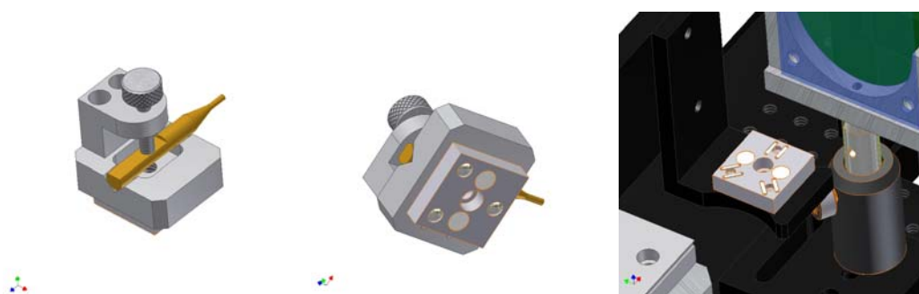
Figure 5 Transfer dop mounted in vee-block (left), magnetic base (middle), and kinematic seat for repeatable locating (right). The dop shown is approximately 50 mm in length and 6.3 mm in diameter.
