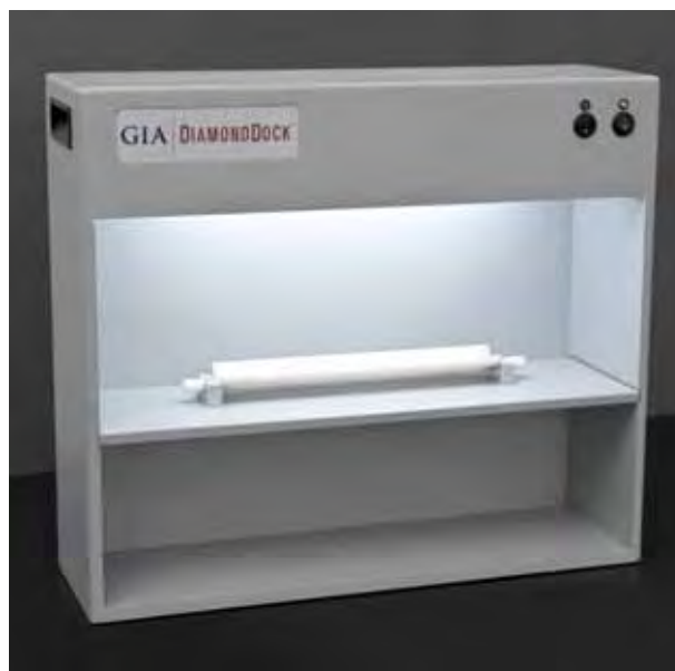
Figure 7. This viewing box, the DiamondDock, provides a good surround for making visual comparisons of diamonds, both for color grading D-to-Z stones and observing round brilliant cuts. When the raised platform is inserted in the box as seen here, a viewing tray of master diamonds is at the appropriate height for color grading. When the platform is removed (and the auxiliary LED lights turned on), cut can be observed with the diamonds placed in a tray on the base of the unit. The box measures about 18 in. high × 21 in. wide × 6½ in. deep (45 × 52.5 × 16.25 cm). Photo by Robert Weldon.
