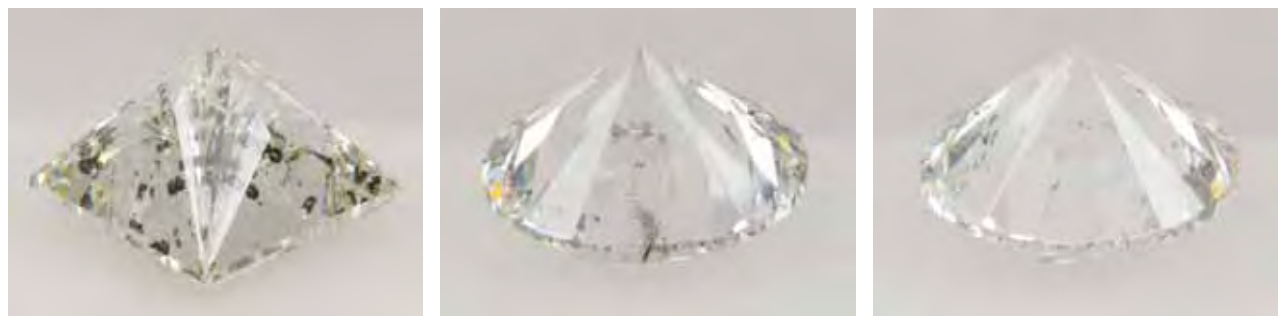
Figure 18. When the grader observes the overall blend of color, the extensive inclusions in the diamond on the far left will become part of the observation and ultimately affect the final grade. When the included area is very limited, as in the diamond in the center, the stone is positioned (far right) to minimize the visual impact of the inclusions on the final grade. Photos by Jian Xin Liao.
