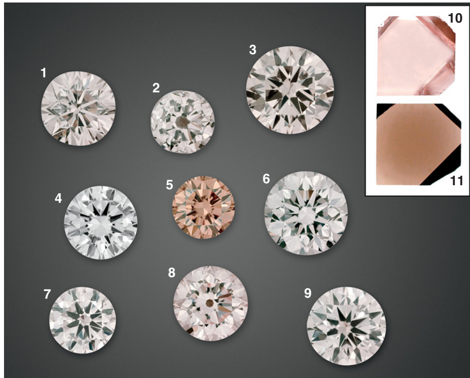
Figure 1. The 11 CVD synthetic diamond samples examined for this study are shown here in their initial “stable” state (i.e., before exposure to heat or a UV lamp). The numbers on the nine round brilliants (0.40–0.92 ct) and two tabular plates (0.22 and 0.35 ct) correspond to the sample numbers used in table 1 and throughout the article. Composite photo by R. Khan.
