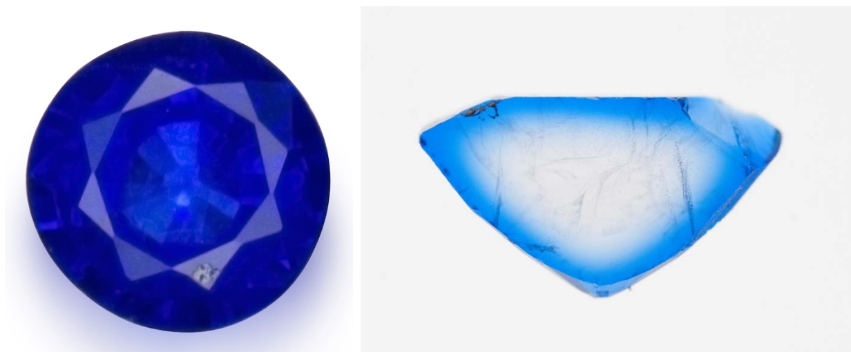
Figure 1: A faceted Co diffused spinel and a cross section through another sample revealing the considerable depth of penetration.
