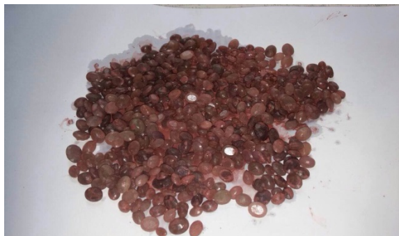
Figure 7: A group of spinels shown here as "coated and ready for the Co diffusion process" (Photo © T. Charasaiya).
