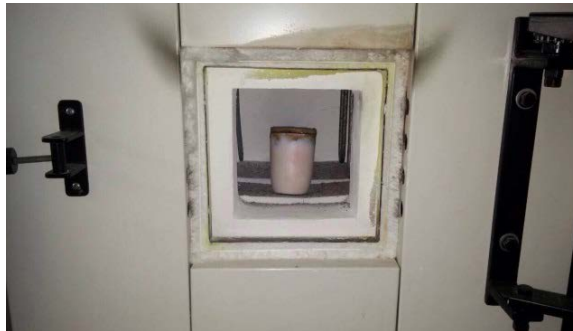
Figure 5: Mr. Thamrong Charasaiya's furnace showing a crucible he uses during the Co diffusion process (Photo © T. Charasaiya).
