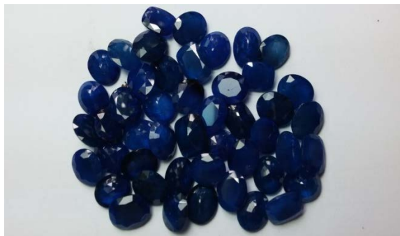
Figure 9: Co diffused spinel after repolishing and ready for the market (Photo © T. Charasaiya)
