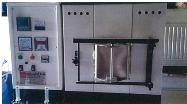
Figure 4: Mr. Thamrong Charasaiya's furnace used for the Co diffusion process. (Photo © T. Charasaiya)
