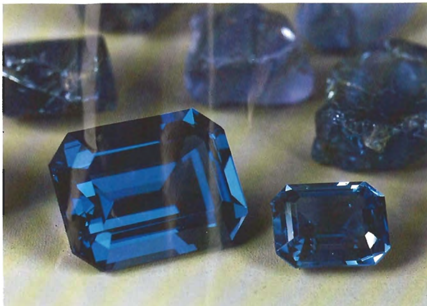
Figure 1. Two natural spinels (5.30 ct and 1.37 ct, respectively) that have the intense blue color normally associated with cobalt-doped synthetic spinel. Photo by Michael Havstad.
