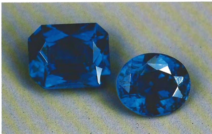
Figure 13. Two spinels of a similar, intense blue. The 1.88-ct stone on the left is a flame-fusion synthetic, while the 1.40-ct one on the right is natural. The spectral curves for these stones (types III and I, respectively; see figure 12) show similarity in the positions and strengths of their absorption bands in the region above 500 nm. However, recognition of the A, B, and particularly the C bands at shorter wavelengths in the natural stone provides a means for distinguishing it from its synthetic counterpart. Photo by Michael Havstad.
