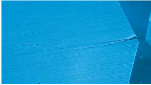
Figure 2. The use of reflected light (especially fiber-optic illumination) can help determine the length of a surface-reaching fissure that may be difficult to see because of the clarity enhancement. Photomicrograph by John I. Koivula; magnified 20x.
