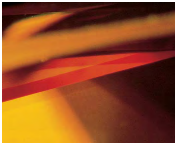
Figure 4. The color zoning characteristic of cyclotron irradiation in diamond follows the crown facets at a shallow depth below the surface of the stone. Photograph by Robert E. Kane; magnified 40×.
