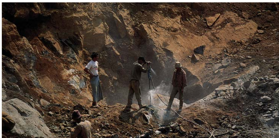
Figure 6. Once a dike is exposed at Tawmaw, jackhammers are needed to break the jadeite apart. Photo © Richard W. Hughes.
