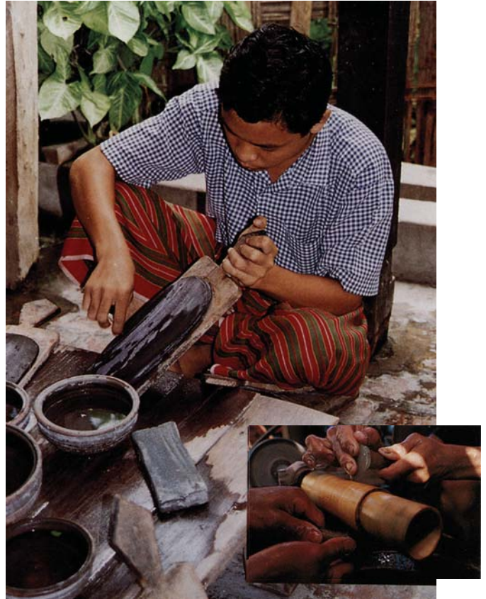
Figure 13. In Mandalay, cutters still use a board coated with a mixture of carborundum (of various grits) and hard wax to shape cabochons (photo by Mark Smith). They then polish jadeite on bamboo lathes, often without any abrasive (inset photo © 2000 Fred Ward).
