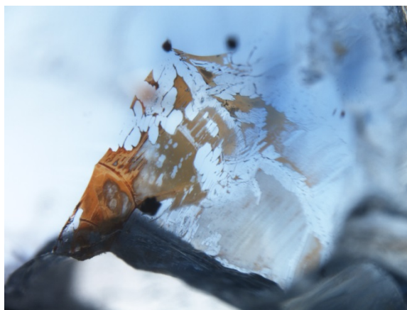
Figure 46: Naturally-healed fissure with orange stains in GIA sample #1945. Darkfield and diffused illumination. FOV 2.7 mm. Photo: C. Khawpong © GIA.
