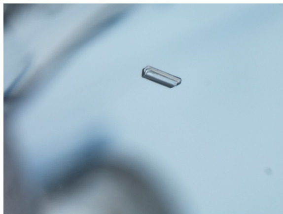
Figure 56: Well-formed feldspar crystal (identified by Raman using the RRUFF database as a reference) in GIA sample #2389. Darkfield and diffused illumination. FOV 1.5 mm. Photo: J. Muyal © GIA.
