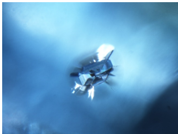
Figure 60: A prismatic zircon crystal (identified by Raman using the RRUFF database as a reference) in GIA sample #9197. Darkfield and fiber-optic illumination. FOV 1.3 mm. Photo: C. Khowpong © GIA.
