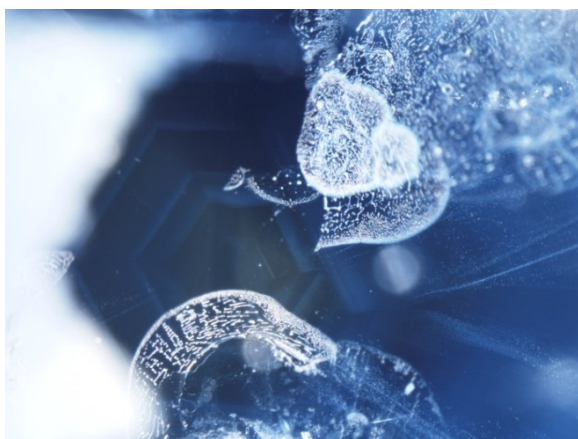
Figure 23: Hexagonal fine grained cloud associated with internal growth features and naturally-healed fractures in GIA sample #7132 using darkfield illumination. FOV 2.5 mm. Photo: J. Moyal © GIA.
