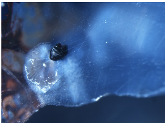
Figure 53: Black unidentified opaque inclusion with decrepitation disk in GIA sample #1945. Fiber-optic illumination. FOV 1.3 mm. Photo: C. Khowpong © GIA.
