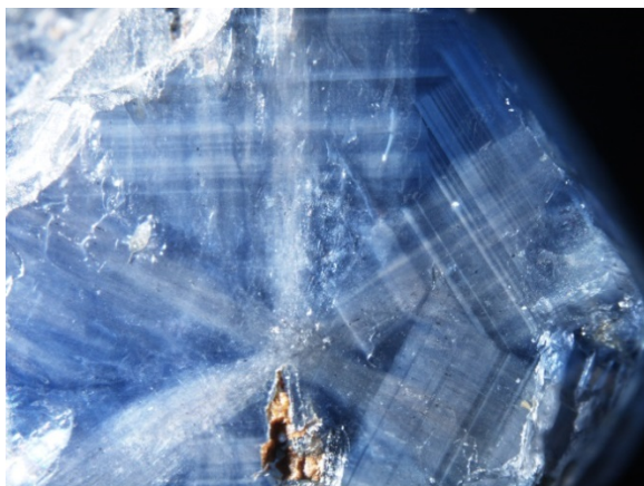
Figure 63: Trapiche pattern and hexagonal zoning in GIA sample #1981. Darkfield and fiber-optic illumination. FOV 4.0 mm. Photo: C. Khowpong © GIA.
