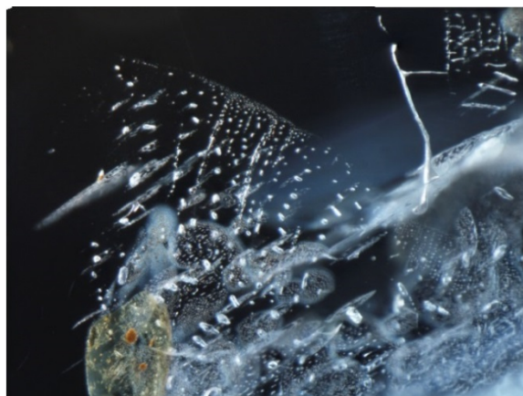
Figure 44: Naturally healed fissures with secondary healed fissures in GIA sample #7164. Darkfield illumination. FOV 1.2 mm. Photo: J. Muyal © GIA.
