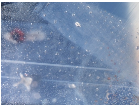
Figure 45: Plane of negative crystals forming a fingerprint in GIA sample #7183. Darkfield and fiber-optic illumination. FOV 1.2 mm. Photo: J. Muyal © GIA.
