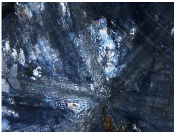
Figure 64: Trapiche pattern and thin films in GIA sample #1981. Fiber-optic illumination. FOV 4.0 mm. Photo: C. Khowpong © GIA.
