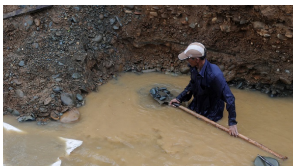
Figure 8: A miner using a long shovel to get gravel from the river bottom. Photo by Wim Verriest-GIA.
