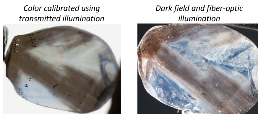
Figure 74: GIA sample #7122-A showing the location of the 25 spots where LA-ICP-MS analysis was conducted on different areas. The photo was color calibrated and captured using transmitted light (left) and bright field and fiber-optic illumination (right). Photo: S. Engniwat © GIA.
