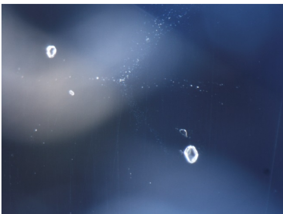
Figure 57: Feldspar crystal with rounded appearance (identified by Raman using the RRUFF database as a reference) in GIA sample #7132. Darkfield illumination. FOV 1.1 mm. Photo: J. Muyal © GIA.
