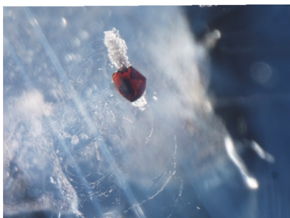
Figure 48: Pyrochlore crystal (identified by Raman using the RRUFF database as a reference) associated with tension haloes and white tail-like inclusions in GIA sample #7183. Darkfield and fiber-optic illumination. FOV 1.1 mm. Photo: J. Muyal © GIA.
