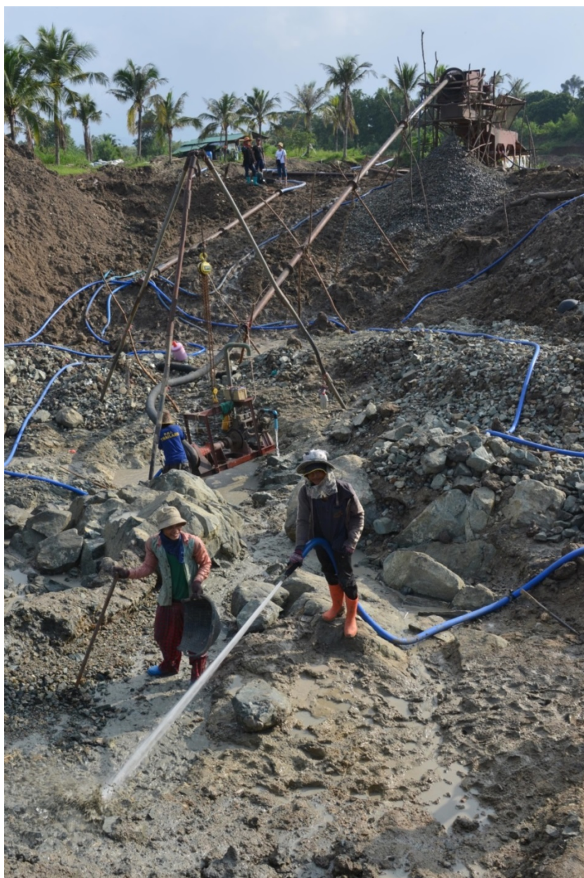
Figure 6: Mining old river deposits near the Pailin River. From bottom to top, we can see: Miner working high pressure waterjet to loosen the gravels; gravel pump to move the slurry; jig to concentrate the minerals. Photo by Vincent Pardieu-GIA.
