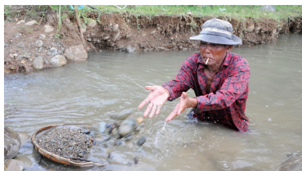
Figure 9: A miner removing the oversized material from his washing screen. Photo by Wim Verriest-GIA.
