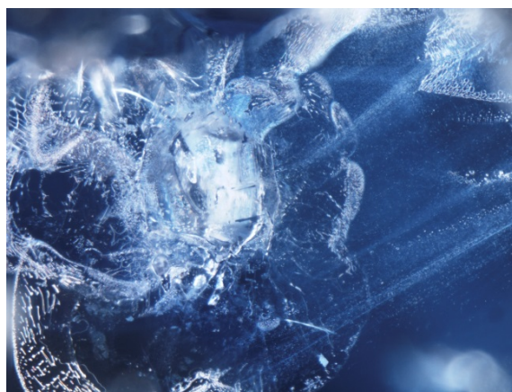
Figure 42: Unidentified inclusion associated with natural-healed fissures in GIA sample #7132. Darkfield and fiber-optic illumination. FOV 2.0 mm. Photo: J. Muylal © GIA.
