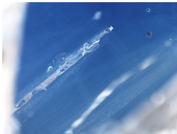
Figure 32: Milky cloud, void like inclusions, and stringers in GIA sample #8502. Darkfield and fiber-optic illumination. FOV 1.7 mm. Photo: J. Moyal © GIA.
