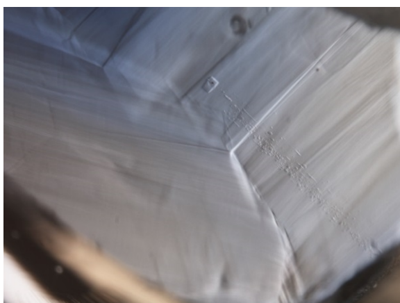
Figure 16: Under brightfield illumination, strong angular growth features are associated with a fine grained cloud showing brownish zoning in GIA sample #2389. FOV 2.5 mm. Photo: J. Moyal© GIA.
