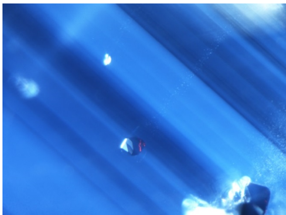
Figure 49: A brownish red pyrochlore crystal with a 'comet tail' in GIA sample #9203. Fiber-optic illumination. FOV 1.1 mm. Photo: C. Khowpong © GIA.
