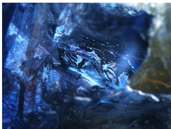
Figure 41: Iridescent natural healed fissure and large reflective fluid inclusions in GIA sample #9210. Fiber-optic illumination. FOV 2.0 mm. Photo: C. Khowpong © GIA.
