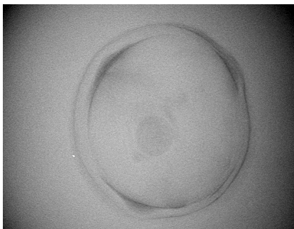
Figure 20: An RTX image of the reported aBCP in Figure 19 a natural pearl 'bead' with a faint rounded, organically dominated, centre. The demarcation between the natural pearl 'bead' and the cultured nacre is clear but the organic gap is 'defused' and has the appearance of a conchiolin accumulation on the edges of the natural pearl 'bead'. Note that no concentric arcs are visible in the cultured nacre.
