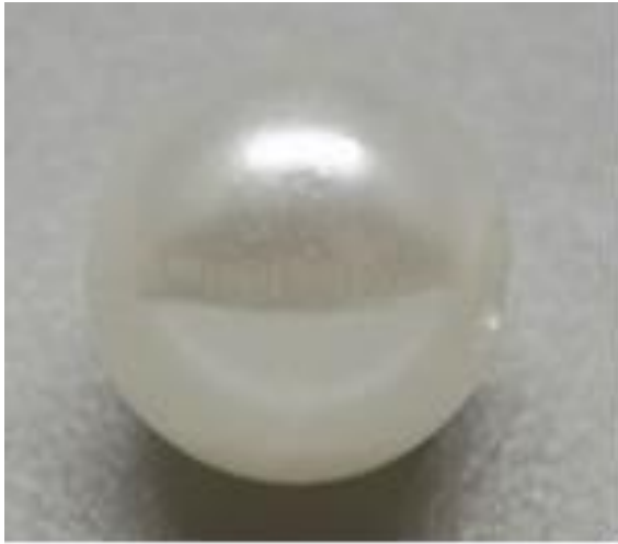
Figure 96: A small 'drilled' plastic imitation pearl weighing 1.14ct used as an atypical 'bead' in 'bead' culturing experiments, see Figure 98, Figure 95 and Figure 97.
