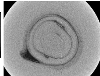
Figure 18: A slice from the \mu CT scan of the reported aBCP in Figure 16 showing the natural pearl used as a 'bead' with a higher definition of the demarcation between the natural pearl 'bead' and the cultured nacre and the organic tail often observed in bead-cultured pearls.
