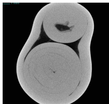
Figure 33: A slice from the \mu CT scan of the reported aBCP in Figure 31 showing the defined structures and demarcation of two 'beads' that are freshwater non-bead cultured pearls.
