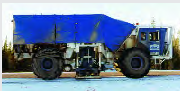
Figure B-2. Vibrator trucks—typically three or more in tandem—are commonly used as a source of energy for seismic-reflection work. Each of these trucks vibrates a signal of known frequency and energy for several seconds. These signals travel into the Earth until they are reflected back to the surface by a rock layer. Photo courtesy of K. W. Hall.
