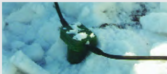
Figure B-3. Geophone sensors, each about 4 cm across the top, are placed on the ground surface to record the vibrations returned from beneath the surface. Photo courtesy of K. W. Hall.
