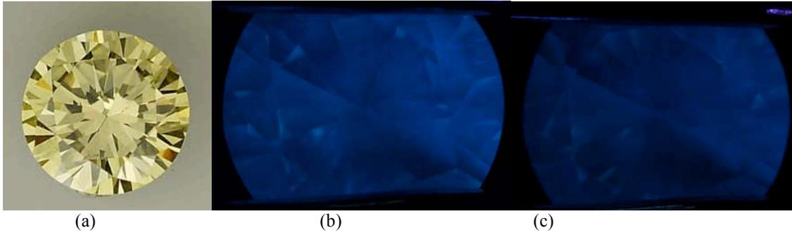
Figure 2. This 0.15 ct type IaA Fancy Intense yellow HPHT-treated diamond (a) displayed faint concentration at the facet junctions when exposed to 100-watt long-wave UV (b), which would alter or disappear when the stone was tilted (c).
