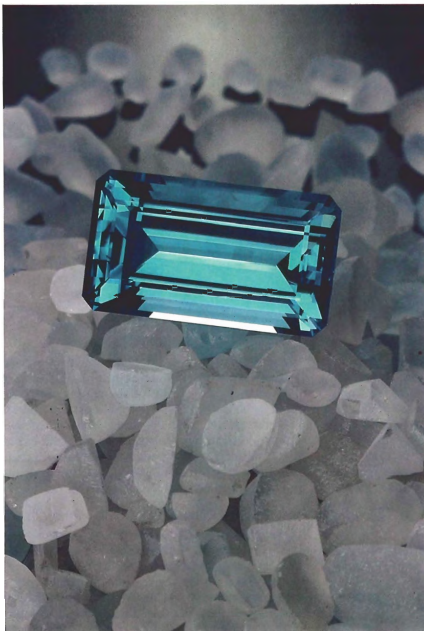
Figure 1. This 57.3-ct topaz derives its color from irradiation (in a linear electron accelerator) and subsequent heat treatment. It originally resembled one of the white topaz preforms on which it sits. Stones courtesy of P. Flusser, Overland Gems, Los Angeles, CA; photo © Tino Hammid.
