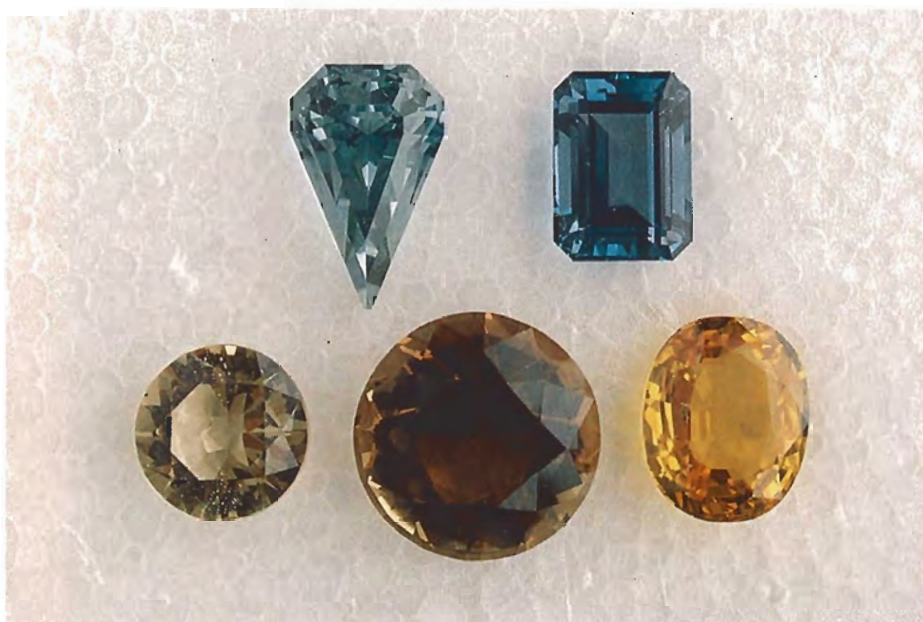
Figure 2. A natural-color blue topaz (left) is notably lighter than its electron-irradiated counterpart (right). Although a wide variety of yellow to brown colors occur naturally or are produced by treatment, the two shades of brown produced by a short dose of gamma rays in the stones on the bottom left provide an interesting comparison with the natural-color yellow topaz on the bottom right.
