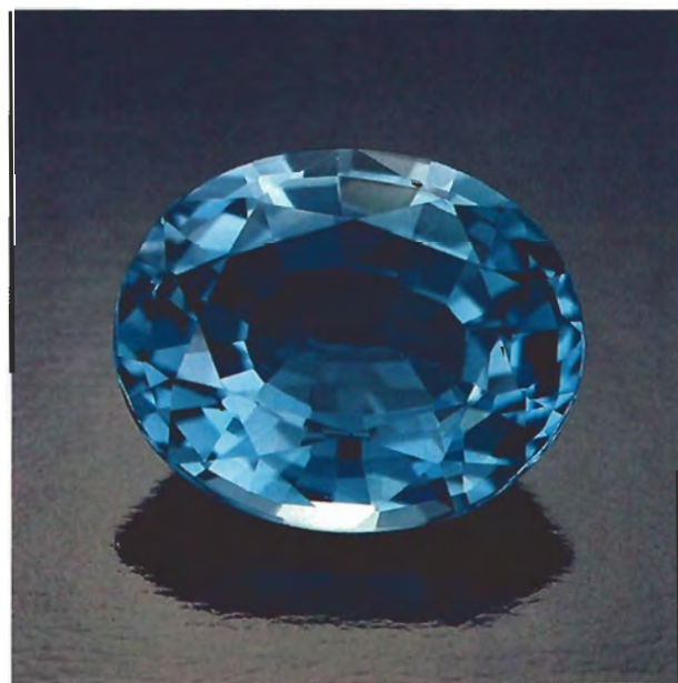
Figure 4. This 6-ct topaz illustrates the "steely" blue color that is often produced in stones subjected to gamma or neutron irradiation.
