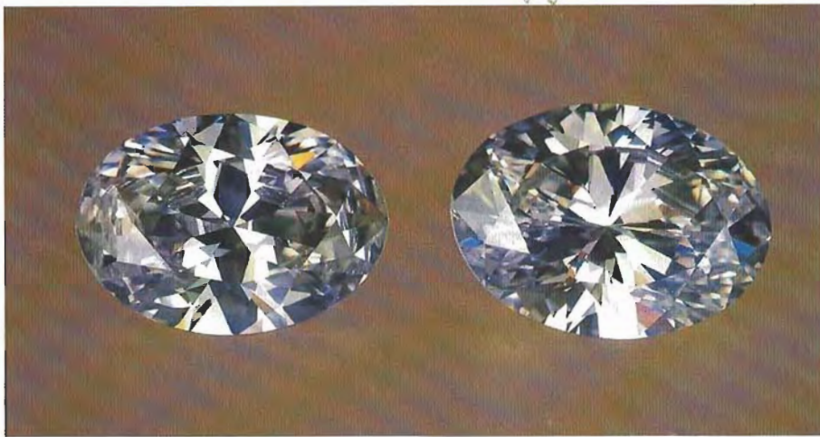
Figure 2. Left = standard oval cut in cubic zirconia, 10.44 ct (note the "bow-tie" effect); right = Watermeyer split-facet oval cut in cubic zirconia, 11.34 ct. Photo by Tino Hammid.
