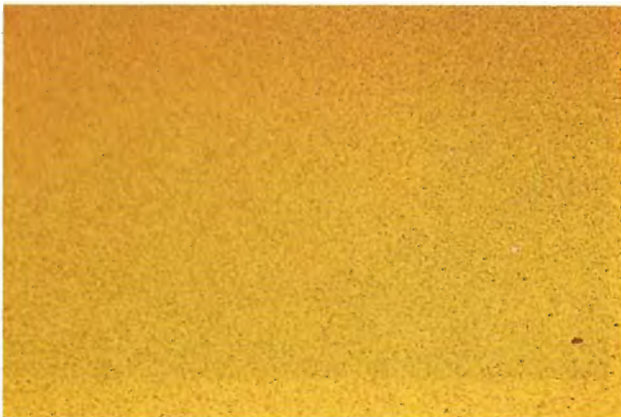
Figure 6. With Nomarski differential interference contrast, the graininess of the surface of the synthetic diamond thin film is readily apparent (left). The only observable features on the surface of the table of the natural cut diamond (right) are grain lines. Photomicrographs by John I. Koivula; magnified 80 \times .
