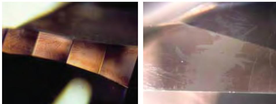
Figure 6. The diamond on the left proved to be a cape stone with a pink coating on the girdle. Note the iridescence and irregular surface features. At right, scratches in the pink coating on this stone are also indicative of this treatment. Photomicrographs by Andrew Quinlan, left (magnified 63×), and Wuyi Wang, right (100×).
