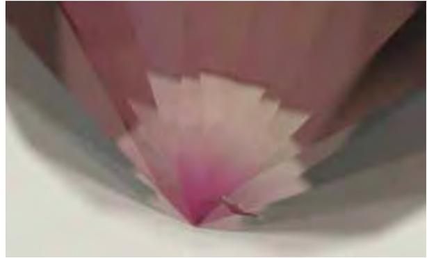
*Figure 9. Lower-energy electron irradiation in a linear accelerator can create a thin layer of color beneath the pavilion facets which, because of internal reflections within the diamond, also appears as a concentration of color at the culet of the stone. In this instance, the color concentration is rather intense, which would not be the case if the thin layer of induced color was less saturated. Photomicrograph by Wuyi Wang; magnified 5×.*
