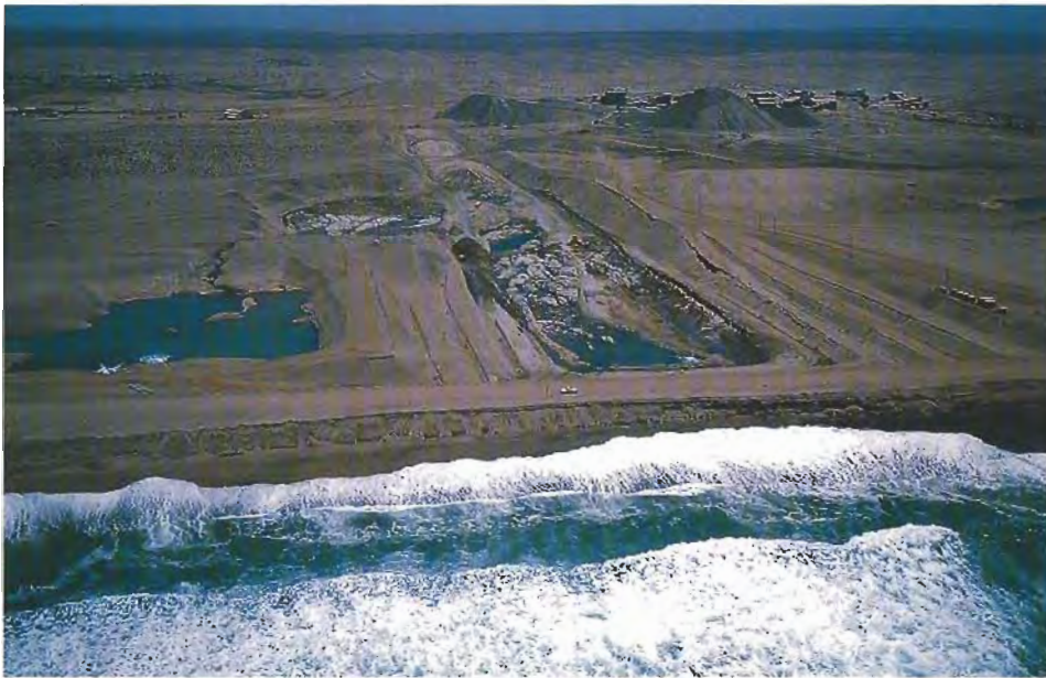
Figure 19. By building huge walls of sand to keep back the sea, CDM has mined vast tracts in Namibia that were once the sea floor. Photo courtesy of De Beers.
