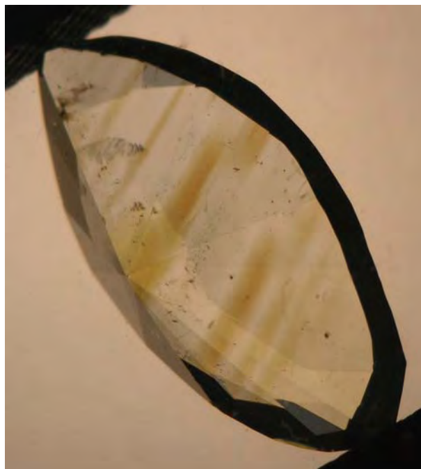
Figure 4. This 1.93 ct chameleon diamond from the Classic group was the only sample that showed distinct color banding. Photo by T. Hainschwang.
