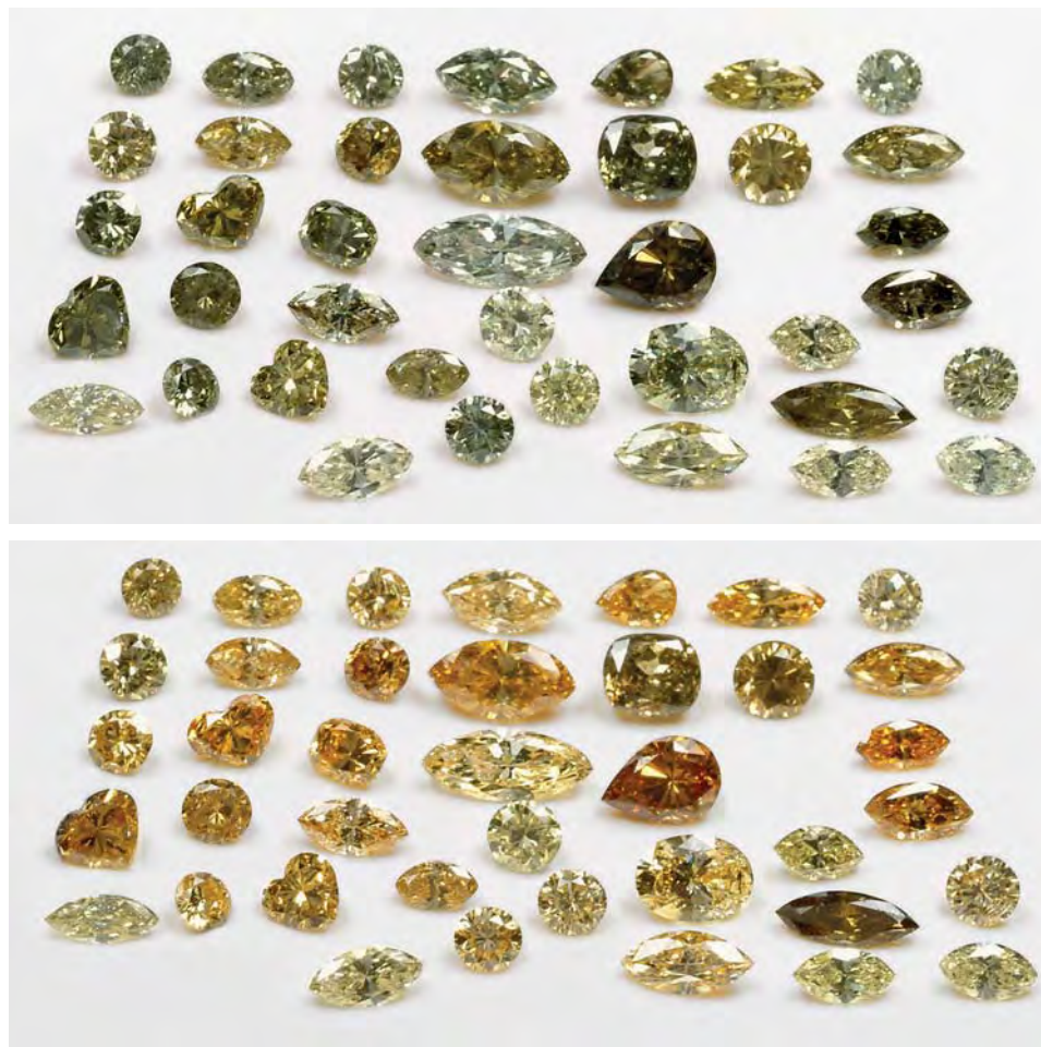
Figure 3. The collection of 39 chameleon diamonds (0.29 to 1.93 ct) is shown at room temperature (top) and when heated to 150°C (bottom). Photos by Julia Kagantsova, EGL.
