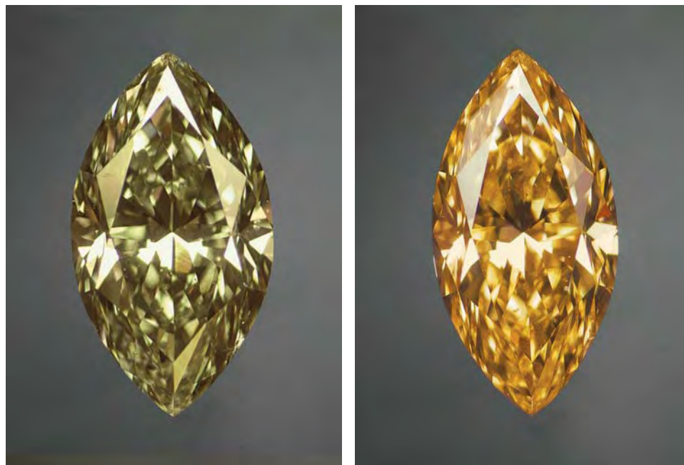
Figure 1. One of the more spectacular chameleon diamonds examined for this study was this 1.01 ct marquise diamond, shown at room temperature (left) and at approximately 150°C (right). Photo by T. Hainschwang.
