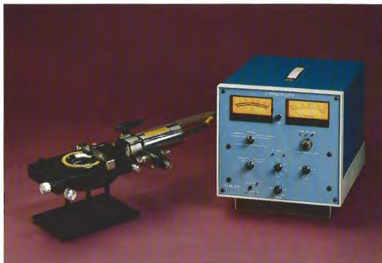
Figure 3. The Luminoscope, manufactured by Premier American Technologies Corp., consists of two parts: On the left is the vacuum chamber and electron "gun," and on the right is the power supply and control unit. Diamonds will emit visible cathodoluminescence when they are bombarded by the electron beam in the vacuum chamber. Photo courtesy of Premier American Technologies Corp., Bellefonte, Pennsylvania.
