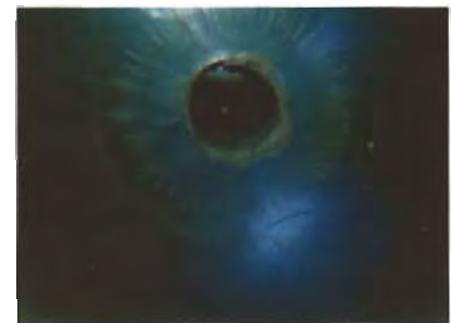
Figure 12. The drill hole in one of the cultured pearls in figure 11 shows the thin nacre and the plastic binding agent which apparently melted from the heat of drilling. Magnified 15×.
