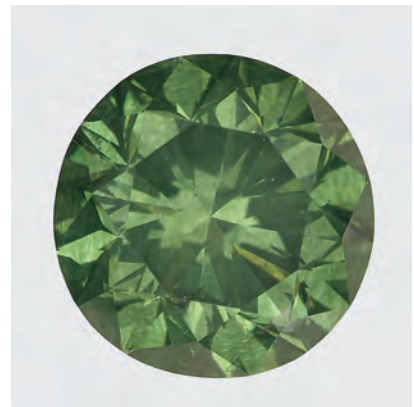
Figure 10. This 3.17 ct round brilliant cut diamond owed its Fancy Deep green color to irradiation with radioactive salts.
