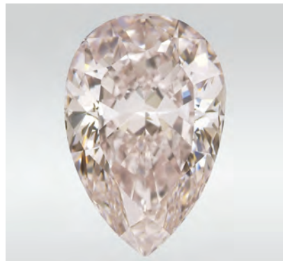
Figure 3. This 20.32 ct pear-shaped diamond was color graded as Fancy pink. Advanced testing suggested that its strong pink color was enhanced by HPHT treatment.
