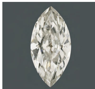
Figure 19. This 2.16 ct marquise ( 13.42 \times 6.73 \times 3.94 mm) is the largest CVD synthetic diamond tested by GIA. It had J/K color, with a brownish tint.
