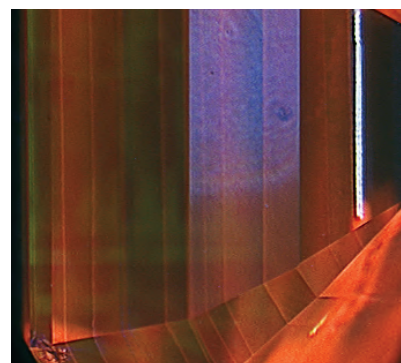
Figure 17. DiamondView imaging showed banded red fluorescence with a striated pattern, typical of CVD synthetic diamonds.
