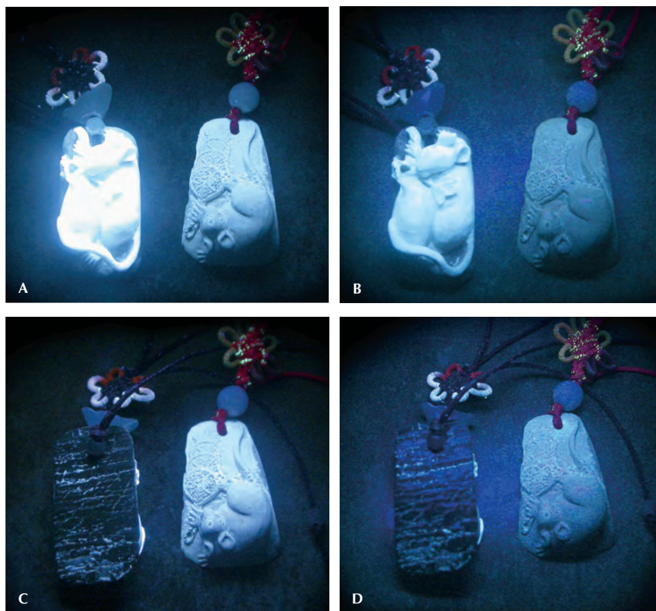
Figure 4. These photos show the fluorescence reaction of mammoth ivory samples M1 and M2 to long- and short-wave UV. The front side of sample M1 is the weakly weathered white layer, which fluoresces stronger bluish white color in long-wave UV (A) and weak bluish white color in short-wave (B). The strongly weathered black layer of sample M1 is inert to both wavelengths (C and D). Sample M2, the semi-weathered brown layer, fluoresces weak bluish white in long-wave UV (A and C) and is inert to short-wave (B and D). Photos by Qinfeng Luo.
