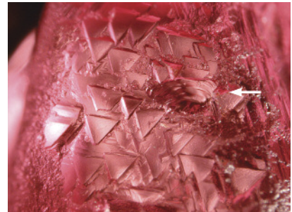
Figure 8. In addition to trigons, the spinel displayed a conchoidal fracture (see arrow), a feature not found in diamond. Magnified 40x.
