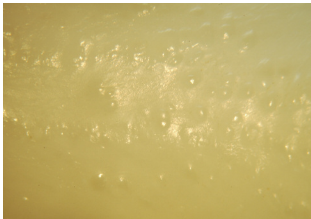
Figure 9. The natural Tridacna pearl showed a characteristic sugary surface texture. Photo by Lai Tai-An Gem Lab; magnified 60x.
