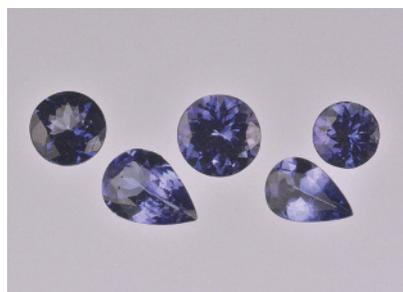
pleochroism. Specific gravity, measured using the hydrostatic method, was 3.37. These properties were consistent with tanzanite.
