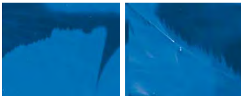
Figure 4. The boundaries between the type zones are linear in some places and jagged in others (left); the type IIa regions in the diamond also show the subtle mottled appearance of “mosaic” dislocations (right).
