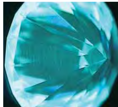
Figure 7. DiamondView imaging of the synthetic diamond shows blue-green fluorescence with yellow-green striations, consistent with reports for HPHT-treated CVD synthetic diamonds.
