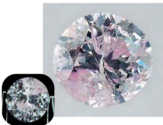
Figure 1. This 0.20 ct “pink” diamond shows uneven color distribution. With strong direct lighting (inset), the pink hue seems to be confined to the two eye-visible fractures, whereas the rest of the stone appears to be near colorless.
