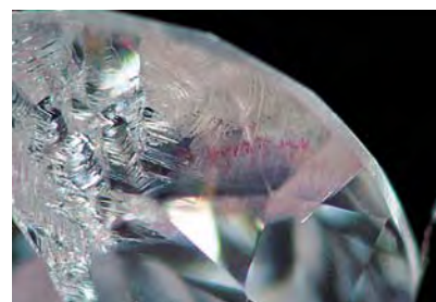
Figure 2. The pink coloring agent is not fully absorbed into the feather and has formed small “beaded” areas of concentrated pink color. Such beaded areas are often seen in clarity-enhanced diamonds. Magnified 45x.
