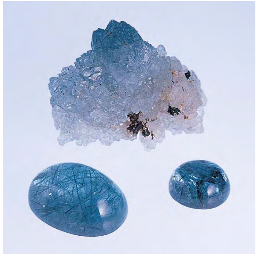
Figure 13. The blue color in both the 30.58 mm crystal group and the polished cabochons of rock crystal quartz (21.76 and 6.96 ct) is caused by inclusions of indicolite.
