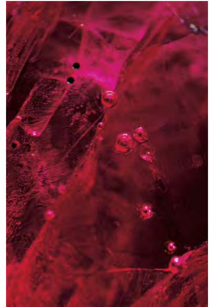
Figure 16. Seen here at 15× magnification are remnants of exploded crystals (brown “balls”), portions of healed fractures, and large gas bubbles—proof that the ruby shown in figure 15 had undergone heat treatment and glass filling.
